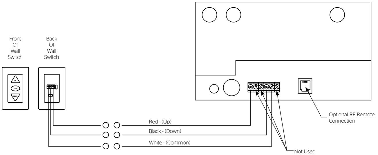
**NOTE:** 20-24AWG wire recommended for connecting wall switch to synchronization controller.
